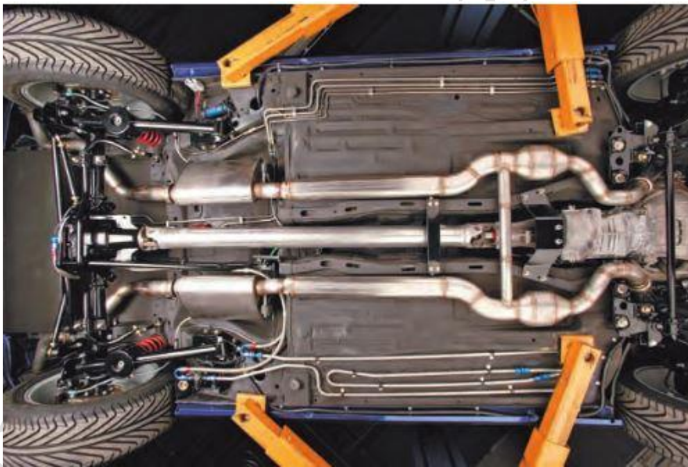
Figure3 –11: In the automotive power train shown, the shaft transmits power from the engine to the rear wheels.
