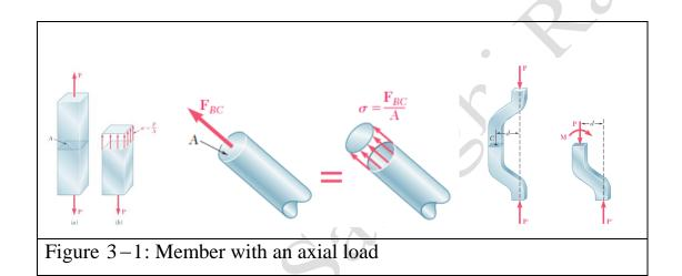
Whether or not the rod will break under the given loading clearly depends upon the ability of the material to withstand the corresponding value  $\frac{F_{BC}}{A}$  of the intensity of the distributed internal forces. It thus depends upon the force  $F_{BC}$ , the cross-sectional area A, and the material of the rod.
