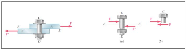
Figure 3-3: bolt subjected to single shear
